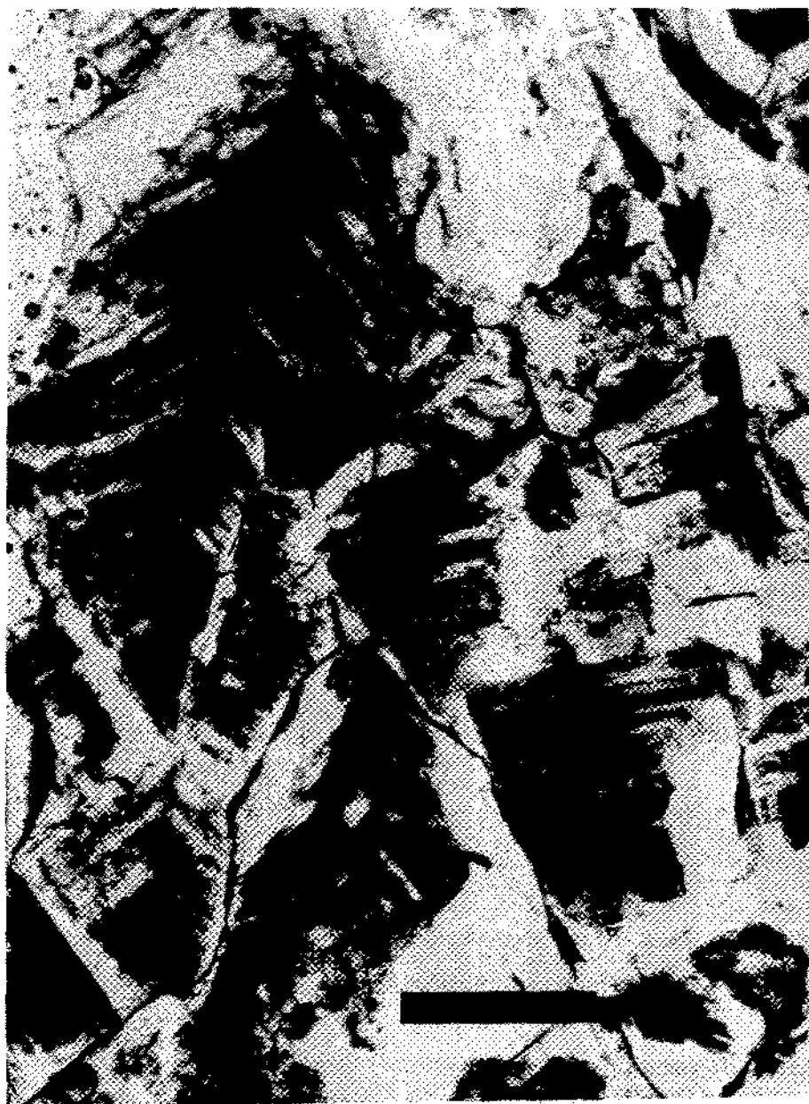
Figure 5. Thin section photograph of vertically oriented halite chevrons (upward directed edges and corners) and corners (upward directed cube faces). Within single crystals, dark bands rich in fluid inclusions alternate with lighter bands containing few fluid inclusions. White areas are clear inclusion-poor halite, usually present as rims on chevrons and corners. Sample from Salado Fm. mud-free halite. Scale bar is 3 mm long.
