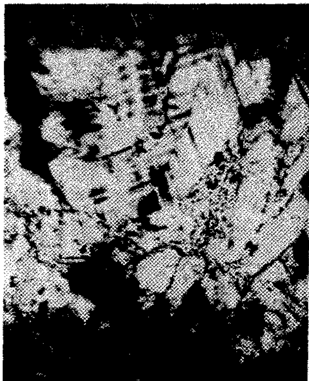
Figure 7. Thin section photograph of fluid inclusion-banded halite crystal with a sharply truncated upper surface. Light halite lamina (1 cm thick) is overlain by gray microcrystalline polyhalite. Sample from Salado Fm. mud-free halite rock.
